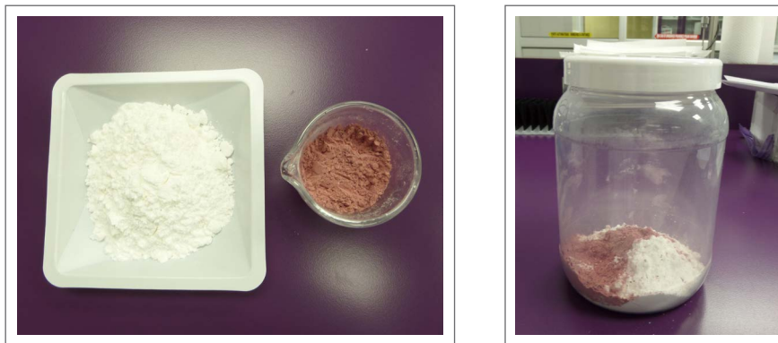
Fig. 3 (left) Lactose and dyed starch, (right) lactose and dyed starch in 1.5 L PET vessel before mixing
