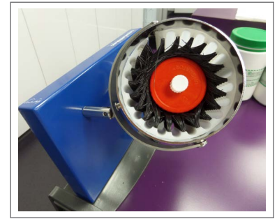
Fig. 5 100 mL Unguator jar secured by brush insert in Inversina Manual Mixer
