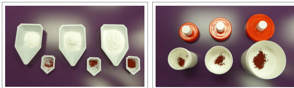
Fig. 4 Methylcellulose and colorant for powder blends in various Unguator jars before mixing
